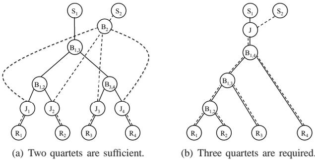
Fig. 3. Two example 2-by- $N$  topologies with  $N = 4$ . In (a),  $\frac{N}{2}$  quartets are sufficient to identify the joining points, *i.e.*,  $(R_1, R_2)$  and  $(R_3, R_4)$ . In (b), more than  $\frac{N}{2}$  quartets are required, *e.g.*,  $(R_1, R_2)$ ,  $(R_1, R_3)$ , and  $(R_1, R_4)$ .
