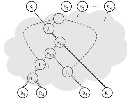
Fig. 1. An example 2-by-4 topology. Solid lines and branching points  $B_{i,j}$ 's depict  $G_{S_1 \times \mathcal{R}}$ .  $J_i$  is a joining point, where  $P_{2i}$  (shown by dashed lines) joins  $G_{S_1 \times \mathcal{R}}$ . An example quartet is the part of the network connecting  $S_1, S_2$  to  $R_1, R_2$ , which is type 1 since both  $J_1, J_2$  lie above the branching point of  $R_1, R_2$  in  $G_{S_1 \times \mathcal{R}}$ , i.e.,  $B_{1,2}$ .
