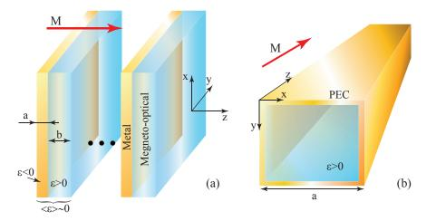
FIG. 2: Schematic of the magneto-active structures exhibiting effective epsilon-near-zero permittivity: a) periodic metal-MO stack, and b) rectangular metallic (PEC) waveguide with a square cross-section. Red arrow shows the direction of magnetization.
