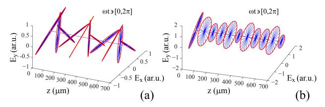
FIG. 4: Electric field distribution along the waveguide at different cross sections and different time frames (Media 2): a) above cut-off at 6.1THz and b) below cut-off at 5.98THz.
