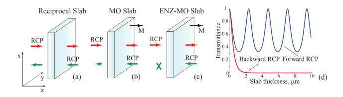
FIG. 1: Schematic of RCP forward and backward transmission through a) reciprocal, b) magnetooptical, and c) magnetically active epsilon-near-zero slabs, respectively. d) Transmittance of the forward and backward RCP plane waves through ENZ-MO slab as a function of the slab thickness.
