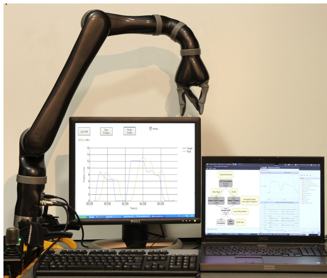
Figure 2: Overview of the experimental setup. OpenViBE (computer on the right side) runs on a linux system to decode intracranial data and send the finger positions to a C# interface (computer on the left side) that translates them into basic commands for the JACO using the API by Kinova. Screen captures of both computers are respectively available as figures 6 and 8.
