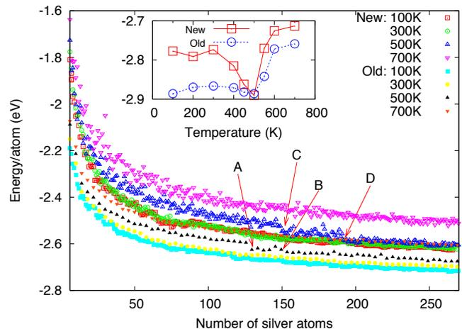
FIG. 7. The evolution of the energy per atom vs Ag cluster size at different deposition temperatures. Open symbols: new parameters, closed symbols: old<sup>43</sup>. The arrows indicates points of energy drops. Inset: temperature dependence of  $e_{\infty}$  (see Eqn. 7).
