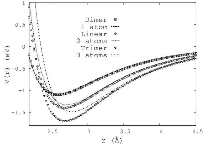
FIG. 5. The validity of the parameterization beyond  $r_c=3.1$  Å. Single atom, two atoms and three atoms are clearly seen to approach the central Ag atom in such a way that the potential of the central atom closely resembles that of an atom in a dimer, a linear chain and in a trigonal arrangement of Ag atoms, respectively.
