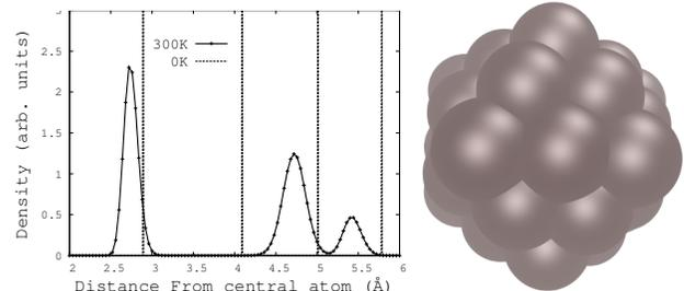
FIG. 6. Left: Density distribution as a function of distance from the central atom of a  $\text{Ag}_{55}$  cluster for the unrelaxed (thin-dotted line) and the MD-relaxed structure at 300 K (full line). The feature at 4.09 Å in the unrelaxed cluster shifts upwards and merges with the feature at 5.0 Å which shifts downwards. Right: Snapshot of MD-relaxed cluster at the end of the 2 ns simulation.
