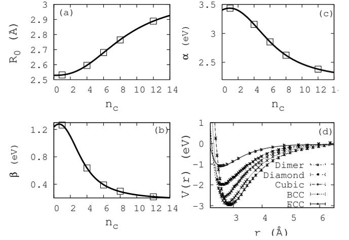
FIG. 3. DFT-parameters of the Gupta potential for the four phases of Ag: face-centered cubic, BCC, simple cubic, Ag in the diamond-like phase and Ag dimer. The fitted potentials are shown in panel (d) and the points are the corresponding DFT binding energies.
