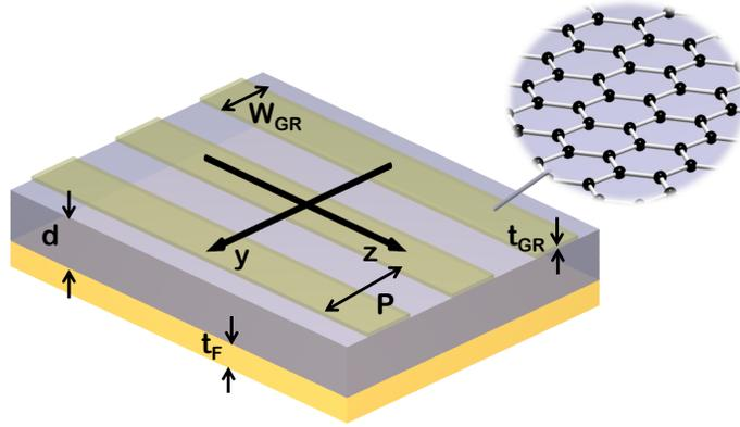
Fig. 1. Schematic of the graphene micro-ribbon perfect absorber. The geometrical parameters of the proposed structure are:  $t_F = 1 \mu\text{m}$ ,  $d = 1 - 100 \mu\text{m}$ ,  $W_{GR} = 1 \mu\text{m}$  and  $P = 2 \mu\text{m}$ . The inset shows the honeycomb microscopic structure of the graphene layer arranged as micro-ribbons.
