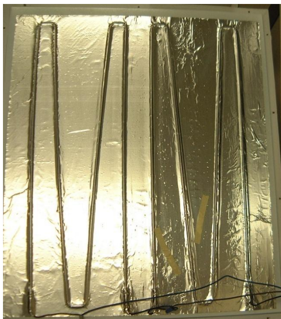
Figure 19. The heating wire inside the door of the Baxter WJ501 incubator.
