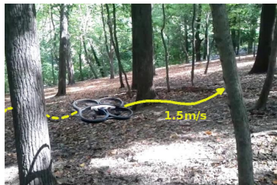
Fig. 1. We present a novel method for high-speed, autonomous MAV flight through dense forest areas. The system is based on purely visual input and imitates human reactive control.
