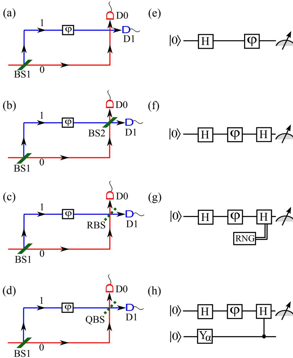
**Figure 6.1:** Different types of Mach-Zehnder interferometer setups (a-d) and equivalent quantum circuits (e-h). BS1 and BS2 are beam splitters,  $\phi$  is phase shifter, D0 and D1 are detectors. RBS is a beam-splitter switched ON or OFF by a random number generator (RNG) and QBS is a beam-splitter which is controlled by a quantum system in superposition. In the quantum circuits,  $H$  is the Hadamard gate and  $Y_\alpha = e^{-i\alpha\sigma_y}$  is used to prepare the state of ancilla qubit.
