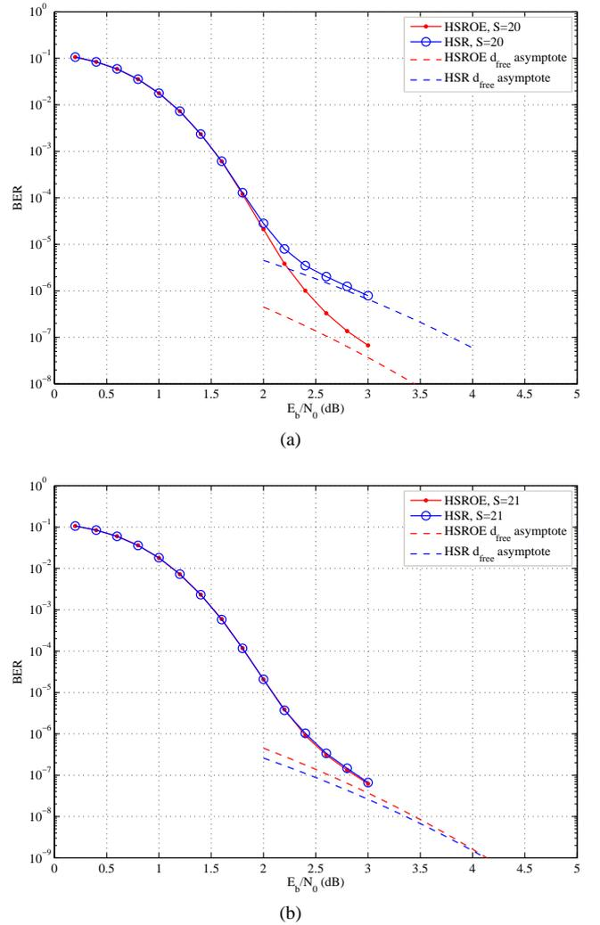
Fig. 2. BER performance of the LTE high-spread random and high-spread random odd-even code ensembles, and corresponding average free-distance ML asymptotes. The  $S$ -parameter takes the values (a)  $S = 20$ , and (b)  $S = 21$ . Interleaver length: 512 bits.
