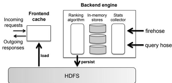
**Figure 4: Architecture of the search assistance engine, consisting of a lightweight frontend serving requests from an in-memory cache and a backend that consumes the firehose and query hose to compute related query suggestions and spelling corrections.**
