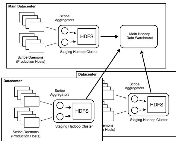
**Figure 2: Illustration of Twitter’s Scribe infrastructure.** Scribe daemons on production hosts send log messages to Scribe aggregators, which deposit aggregated log data onto per-datacenter staging Hadoop clusters. Periodic processes then copy data from these staging clusters into our main Hadoop data warehouse.
