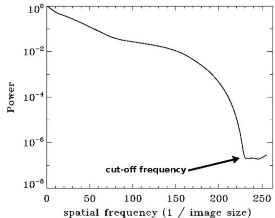
**Fig. 3.** Normalized power spectrum of the 53% SR PSF (Fig. 1 middle left). The diffraction- and noise-limited cut-off frequency was determined to be approximately 230 pixels. The PSF was embedded in an array of zeros to match the size of the science image (512×512 pixels).
