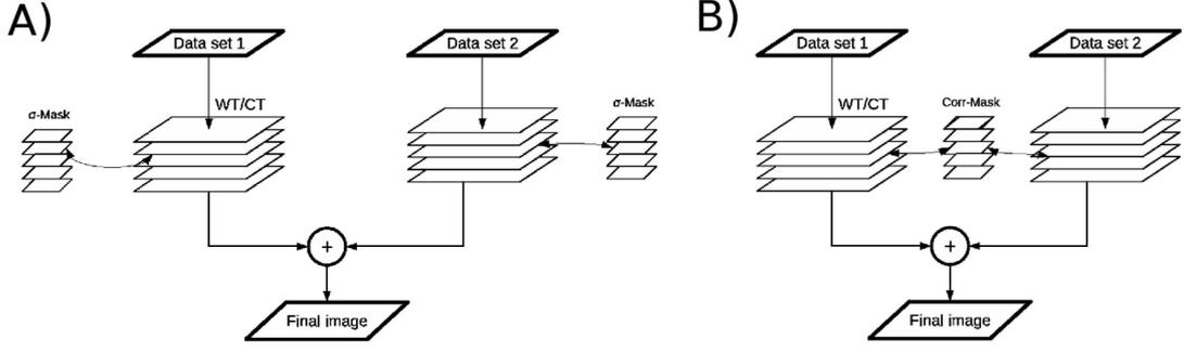
**Fig. 2.** A: A flow graph illustrating the execution of the AWMLE algorithm with the  $\sigma$ -based mask. Datasets are decomposed by WT and each of the resulting planes is *independently* analyzed with the  $\sigma$ -based mask. B: A respective graph for execution with the correlation-based mask. After decomposition the planes are *simultaneously* analyzed with the correlation-based mask.
