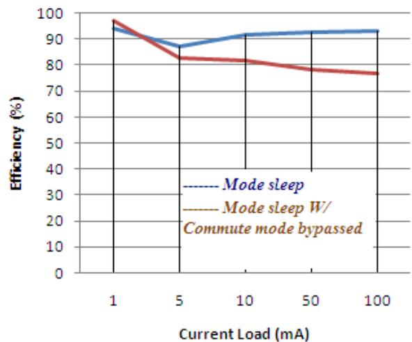
Fig.3.2 efficiency in mode sleep versus current load
