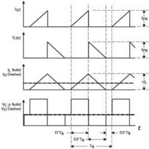
Fig.2.3 Discontinuous-Mode Buck Power Stage Waveforms
