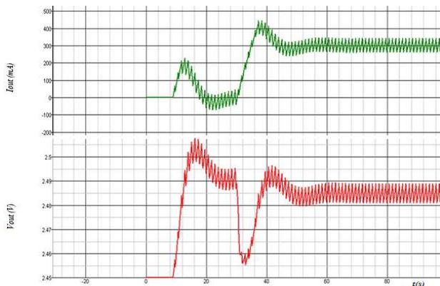
Fig.3.3 output of the proposed buck converter
