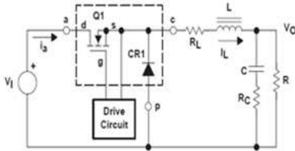
Fig.1.2 Buck power stage Schematic
