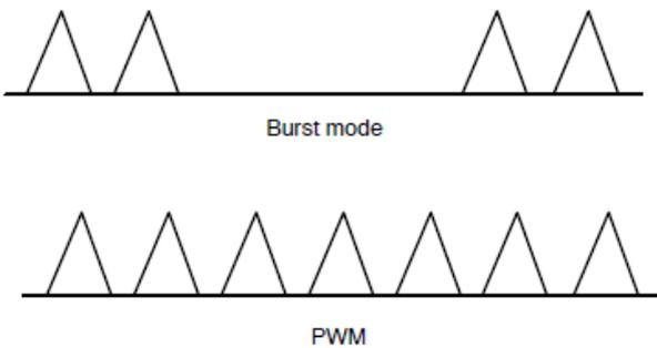
Fig.2.4 DCM Inductor Currents in Burst Mode and PWM Control
