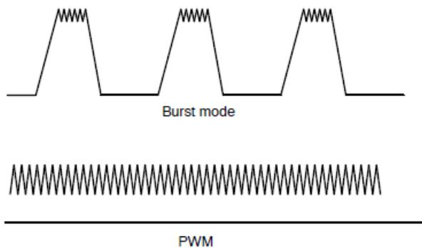
Fig.2.5 CCM Inductor Currents in Burst Mode and traditional PWM Control
