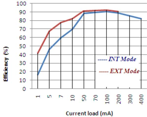
Fig.3.1 efficiency in mode on versus current load
