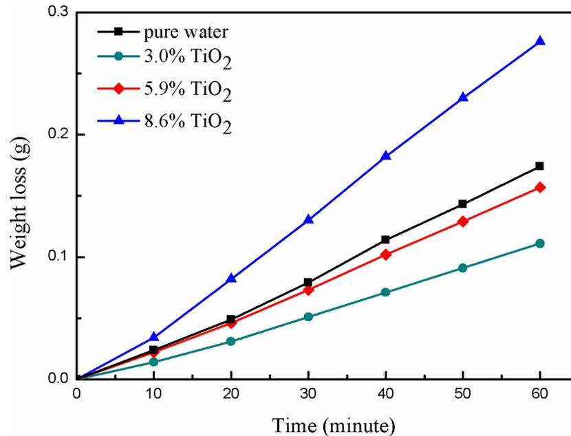
FIG. 6. Weight loss as a function of time for pure deionized water (2 ml) and water (2 ml) dispersed with different amounts of anatase TiO<sub>2</sub> nanoparticles of 25 nm in size. Specified in the graph is the corresponding volume fraction. Environmental temperature: 50 °C; humidity: 20%.
