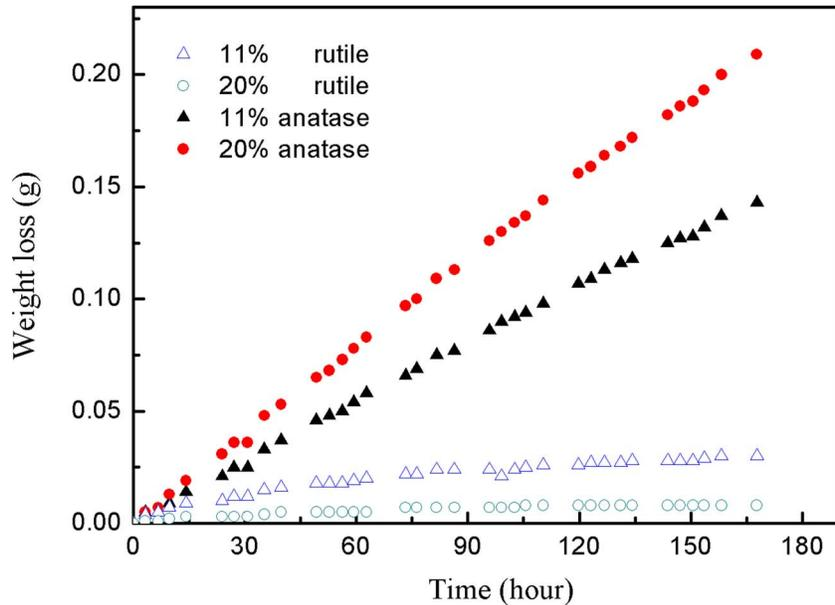
FIG. 3. Comparison of weight losses for the dispersion samples made of silicone oil (2 ml) with anatase and rutile  $\text{TiO}_2$  nanoparticles. Nominal particle size: 10 nm. Specified in the graph are the corresponding volume fractions.
