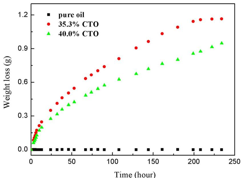
FIG. 1. Weight loss as a function of time for 3 ml (2.91 g) pure silicone oil (square) and for silicone oil plus  $\text{CaTiO}_3$  nanoparticle dispersed systems with a particle volume fraction of 35.3% (circle) and 40.0% (triangle), respectively. Environmental temperature:  $50^\circ\text{C}$ ; humidity: 20%.
