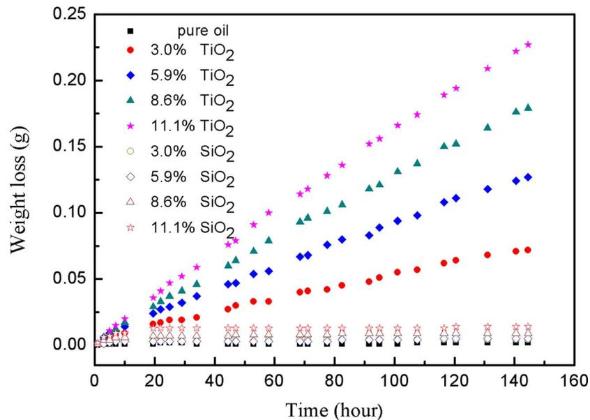
FIG. 2. Weight loss as a function of time for silicone oil (2 ml) dispersed with different amounts of TiO<sub>2</sub> and SiO<sub>2</sub> nanoparticles. Specified in the graph are the corresponding volume fractions.
