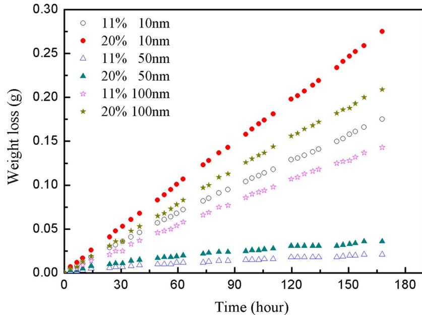
FIG. 4. Comparison of weight loss for the dispersed samples made of silicone oil (2 ml) with anatase  $\text{TiO}_2$  nanoparticles of various sizes. Particle size and the corresponding volume fraction are specified in the graph.
