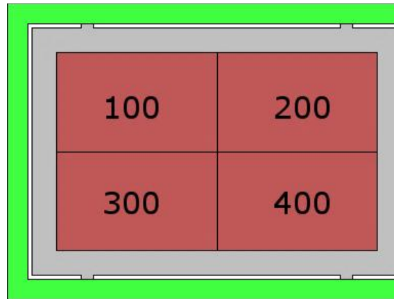
Figure 1: Modified initial spatial pedestrian distribution of IMO's test case 9. Instead of placing initially 250 occupants in each of the four quadrants (the red / dark grey areas in the middle), the initial distribution is chosen to be as shown by the numbers. As the quadrants are areas which by distance can be assigned to one of the four exits, the distribution that results from "everyone to the nearest exit" would be unbalanced and evacuation time would be considerably higher than in the case of balanced initial density. With the surrounding green / dark grey area all four exits are combined to be one, such that there is just one single travel time assessment and the simulated pedestrians implicitly and automatically turn to the right exit (the one which promises smallest estimated individual travel time)
