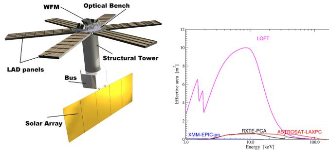
Fig. 1. *Left*: Artist's impression of the LOFT satellite. The SDD of the LAD are placed over the 6 panels extending from the spacecraft optical bench. These panels are stowed during launch and deployed once in space. The WFM is located at the top of the optical bench. *Right*: LAD effective area as a function of the energy (other X-ray astronomy satellites are shown for comparison).
