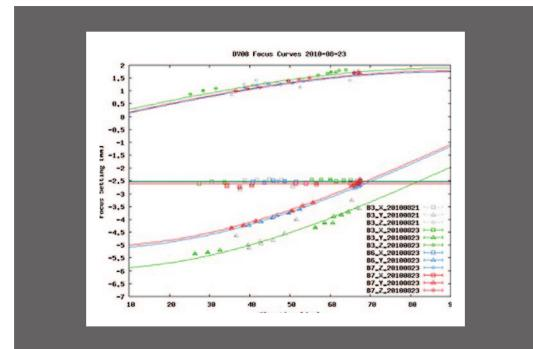
This is a compilation of optimum focus settings (in three different focus directions) for one antenna at various elevations. The results of these measurements are used by the ALMA control software to automatically refocus the antenna during observations.
