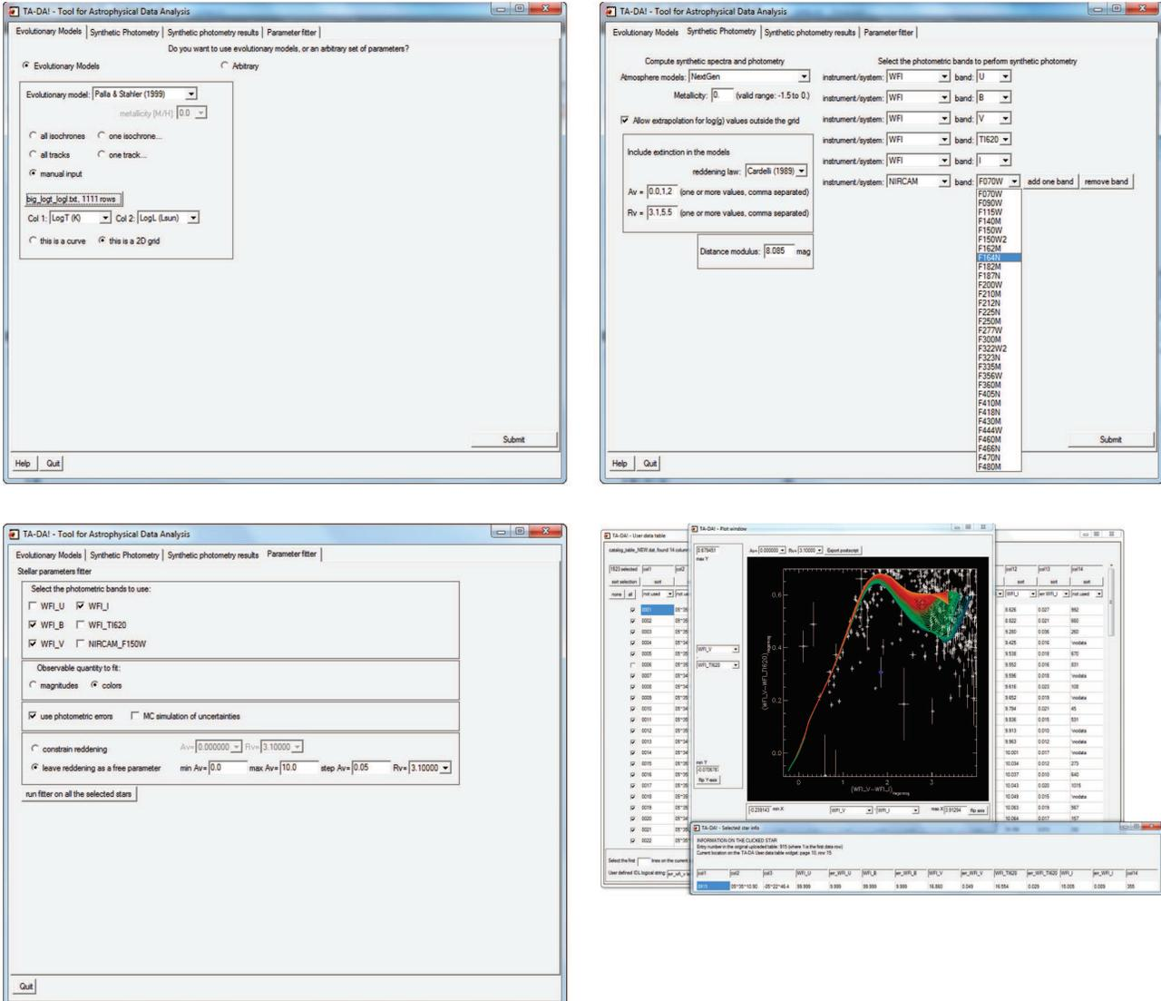
FIG. 1.— Some examples of the graphical user interface of TA-DA: *top left*: the interpolation of evolutionary models or the definition of the model stellar parameters; *top right*: the interface for the synthetic photometry; *bottom right*: the visual inspection of the computed synthetic photometry, the attachment of observed photometry and the selection of sources within the observed catalog; *bottom left*: the interface for the stellar parameter filter.
