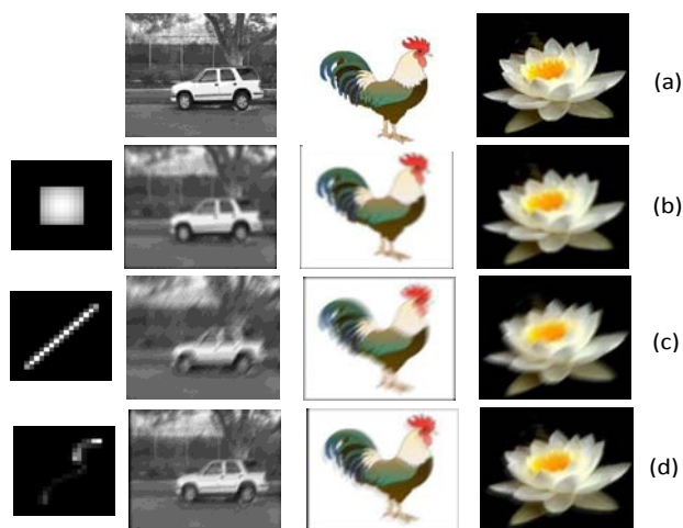
Fig. 2. (a) Sharp images. (b) Gaussian kernel and blurred images. (c) Motion kernel 1 and blurred images. (d) Motion kernel 2 and blurred images.
