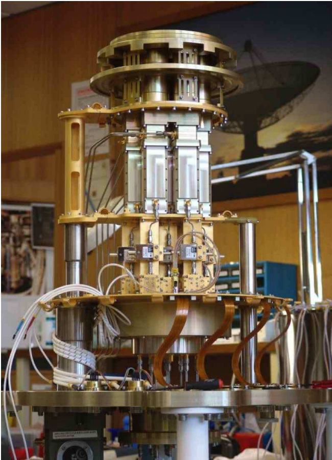
FIG. 1.— The purpose built seven beam Methanol Multibeam receiver.
