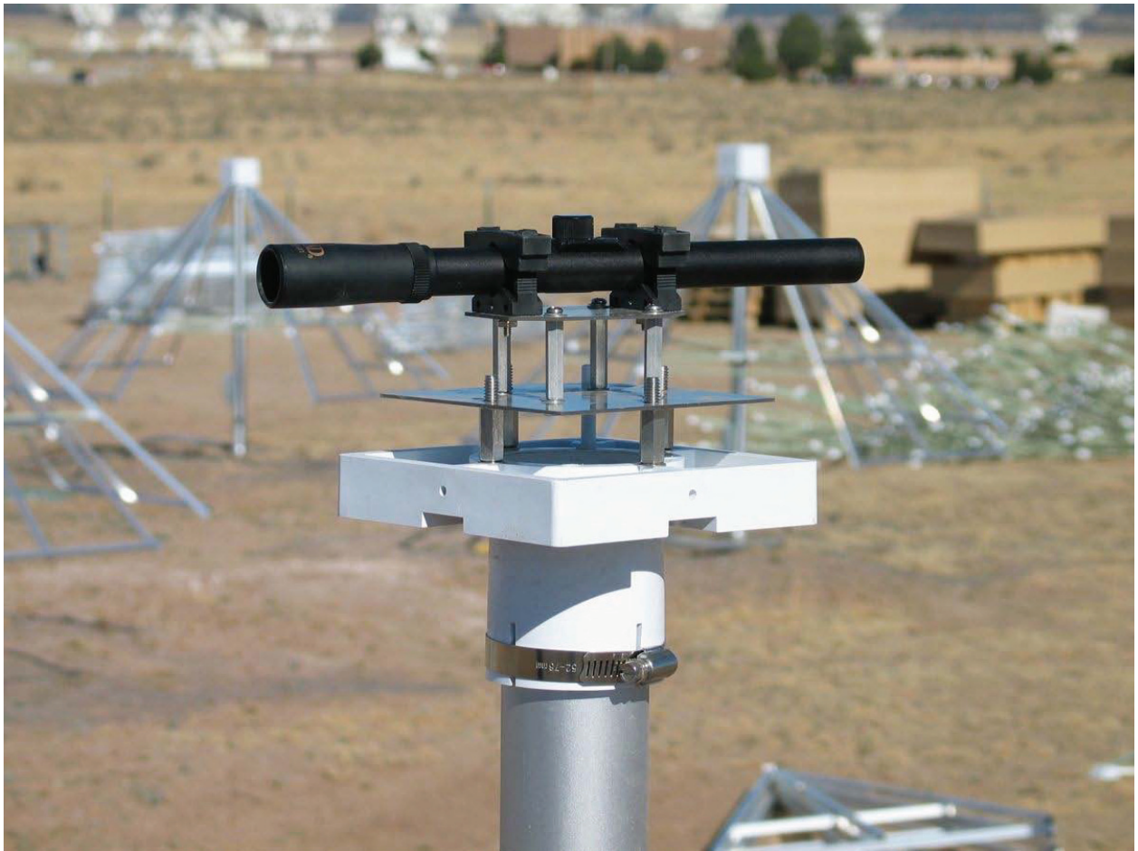
Fig. 10.— STD sighting telescope alignment mechanism used for the LWA1.
