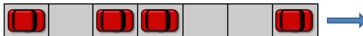
Figure 1. Road setup The road is represented by a periodic boundary 1D lattice divided into L=200 cells. Each cell is either empty or occupied by a single car.
