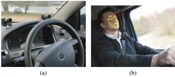
Fig. 4: The eye-tracker Facelab
