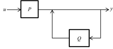
Fig. 4. DSF can be viewed as an interconnection of two systems characterized by the transfer function matrices  $Q$  and  $P$ , where  $Q$  is a hollow transfer function matrix. The transfer function from  $u$  to  $y$  is given by  $G = (I - Q)^{-1}P$ .
