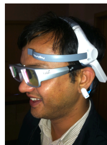
Figure 1. A user wearing the mobile eye tracker and the wearable EEG.
