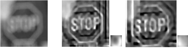
Fig. 6. Non-uniform blur kernels. Left: The observed blurry image. Middle: The deblurred version produced by our algorithm with \alpha = 1000 . Right: The deblurred version produced by our algorithm with \alpha = 4000 .
