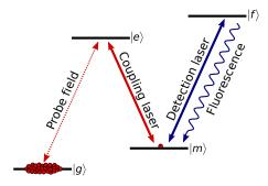
FIG. 1. Principle of the atom-based photon detector as originally proposed [10, 11]. First, an ensemble of identical atoms is prepared in their ground state  $|g\rangle$ . Next, photons in the probe field are converted into collective excitations in the metastable state  $|m\rangle$  with the help of a coupling laser. Finally, the number of collective excitations is probed by collecting fluorescence on the closed transition  $|m\rangle \leftrightarrow |f\rangle$
