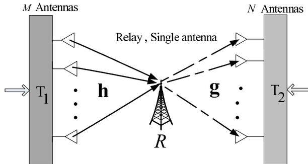
Figure 1: A MIMO cooperative scheme operating in amplify-and-forward (AF) mode with single-antenna relay node
