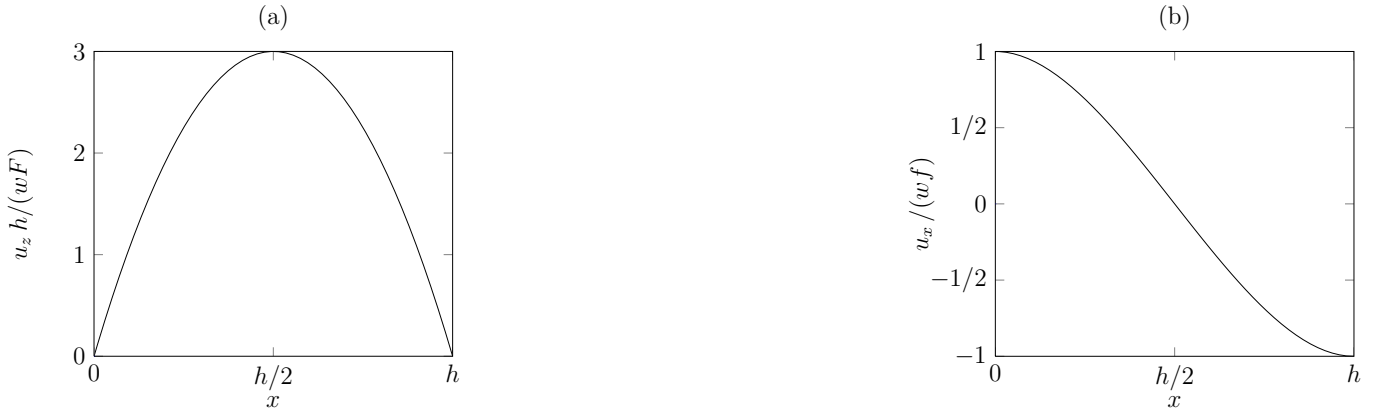
FIG. 3. Flow between parallel porous plates located at x = 0 and x = h with boundary conditions u_x(0) = wf and u_x(h) = -wf . (a) Axial flow velocity u_z given in Eq. (46) plotted as a function of vertical position x . (b) Transverse flow velocity u_x Eq. (45) plotted as a function of vertical position x .
