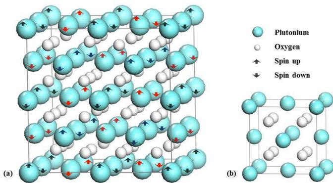
FIG. 1: (a) Atomic structure and magnetic arrangement of  $\alpha$ -Pu<sub>2</sub>O<sub>3</sub> within one unit cell. (b) Atomic structure of the fluorite PuO<sub>2</sub>.
