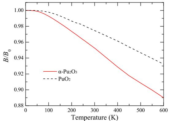
FIG. 4: Temperature dependence of the bulk modulus  $B$  for  $\alpha$ -Pu<sub>2</sub>O<sub>3</sub>. The inset is the ratio of  $B/B_0$  for  $\alpha$ -Pu<sub>2</sub>O<sub>3</sub> and PuO<sub>2</sub>.
