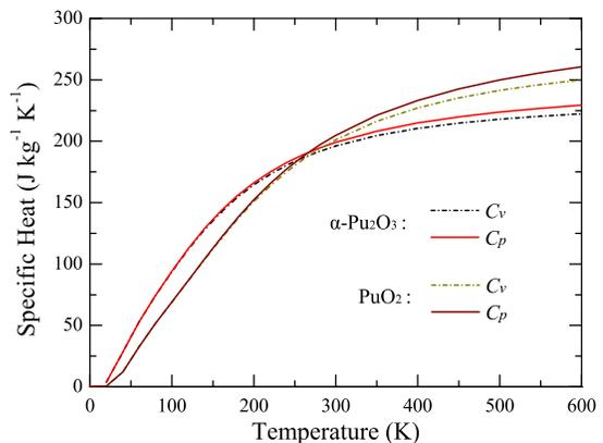
FIG. 5: Heat capacities of  $\alpha$ -Pu<sub>2</sub>O<sub>3</sub> and PuO<sub>2</sub> at constant volume ( $C_V$ ) and constant pressure ( $C_P$ ).
