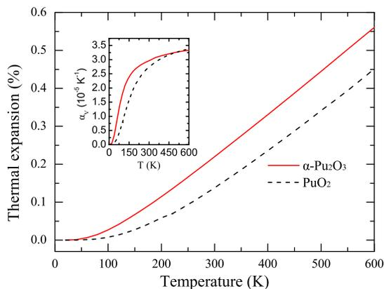
FIG. 3: Temperature dependence of the linear thermal expansion for  $\alpha$ -Pu<sub>2</sub>O<sub>3</sub> and PuO<sub>2</sub>. The inset is the volume thermal expansion coefficient as a function of temperature.
