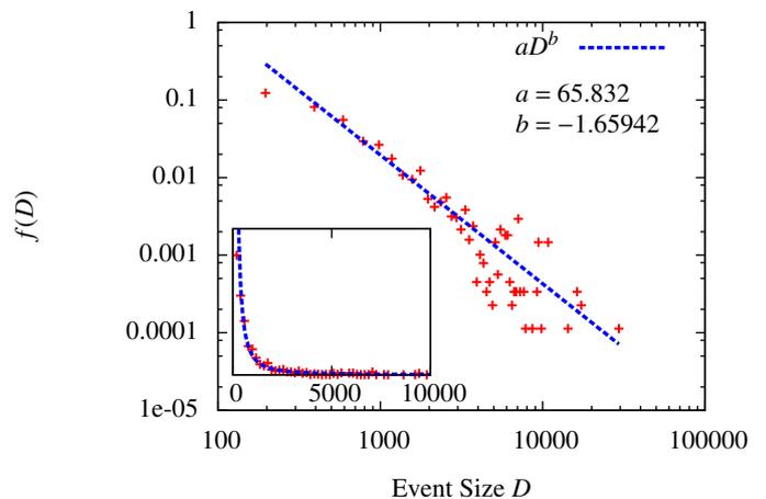
Figure 5: The logarithm of the probability density function  $f(D)$  of the duration as a function of  $\log D$ . The power law fit yields a value for the scaling coefficient of  $-1.659 \pm 0.155$  in the interval  $[200, 3783]$ . The inset exhibits  $f(D)$  as a function of  $D$ .
