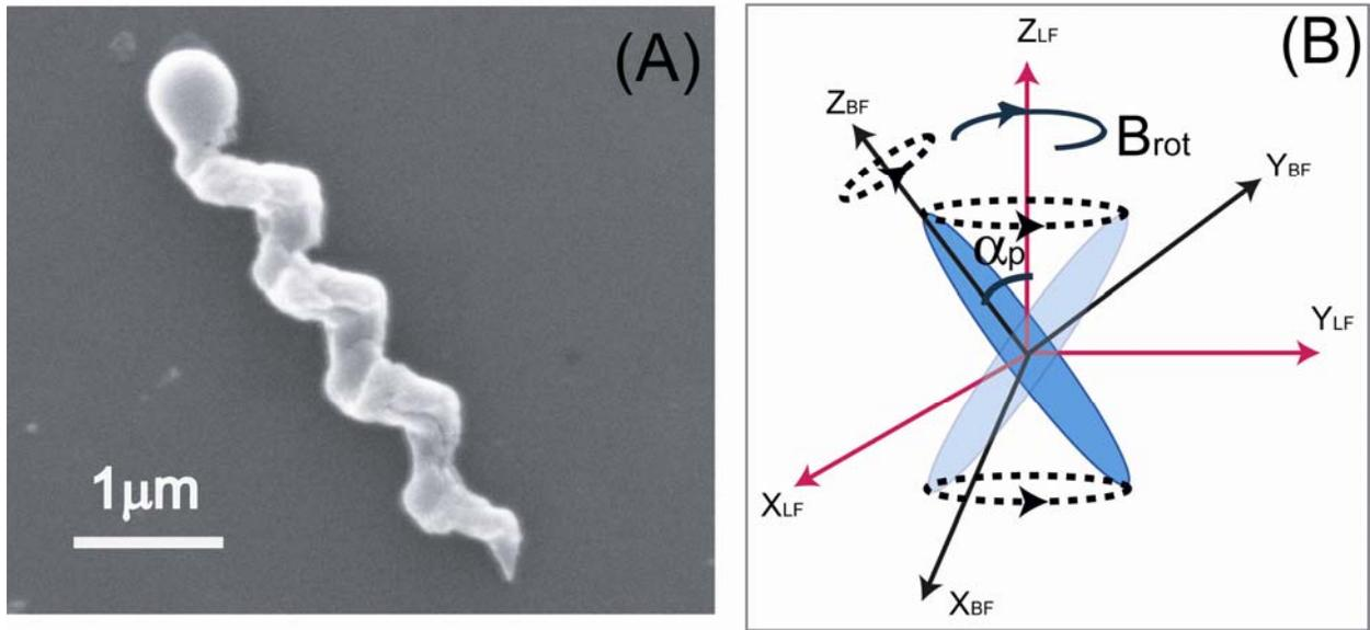
Figure 1 (color online): (A) SEM image of a single nanopropeller. (B) Schematic of the coordinate systems (BF: body frame and LF: laboratory frame) to model the precessional motion (angle  $\alpha_p$ ) of an ellipsoid under a magnetic field,  $B_{rot}$ , rotating in the xy-plane.
