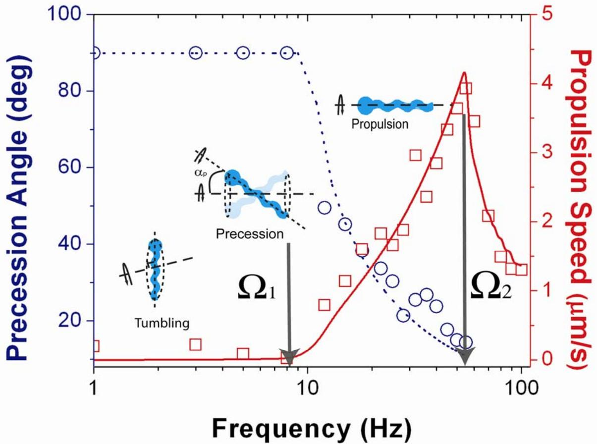
Figure 2 (color online): Experimental data for speed of propulsion (red squares) and angle of precession (blue circles) as a function of frequency for magnetic field of 20 Gauss. Inset schematics show the variety of dynamical configurations. The solid and dotted lines correspond to the propulsion speeds and precession angles of the propeller based on the theoretical model described in the text.
