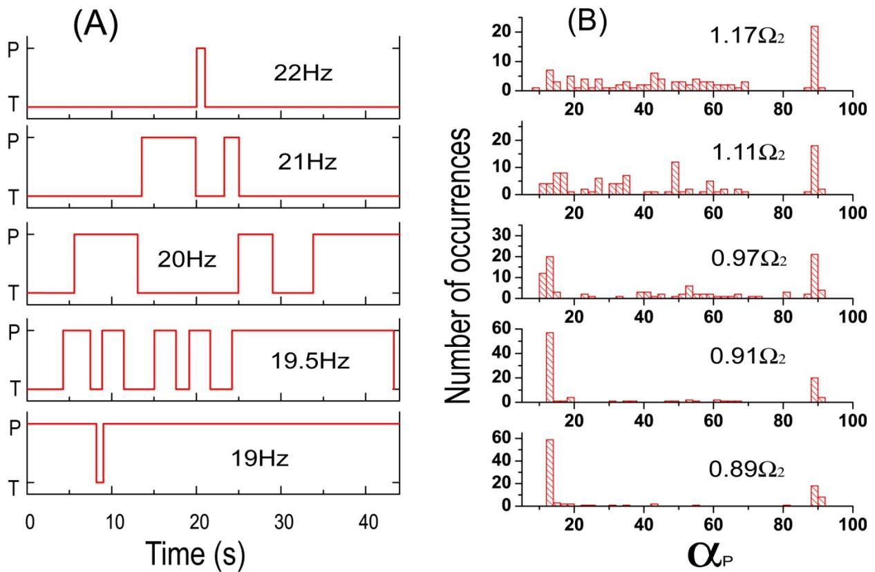
Figure 4 (color online): (A) Experimental: Time series of the dynamical configurations (denoted by “P” for propulsion and “T” for tumbling) at different frequencies. (B) Simulation: Histogram of the steady state precession angles for 100 random initial orientations of the propeller at various frequencies.
