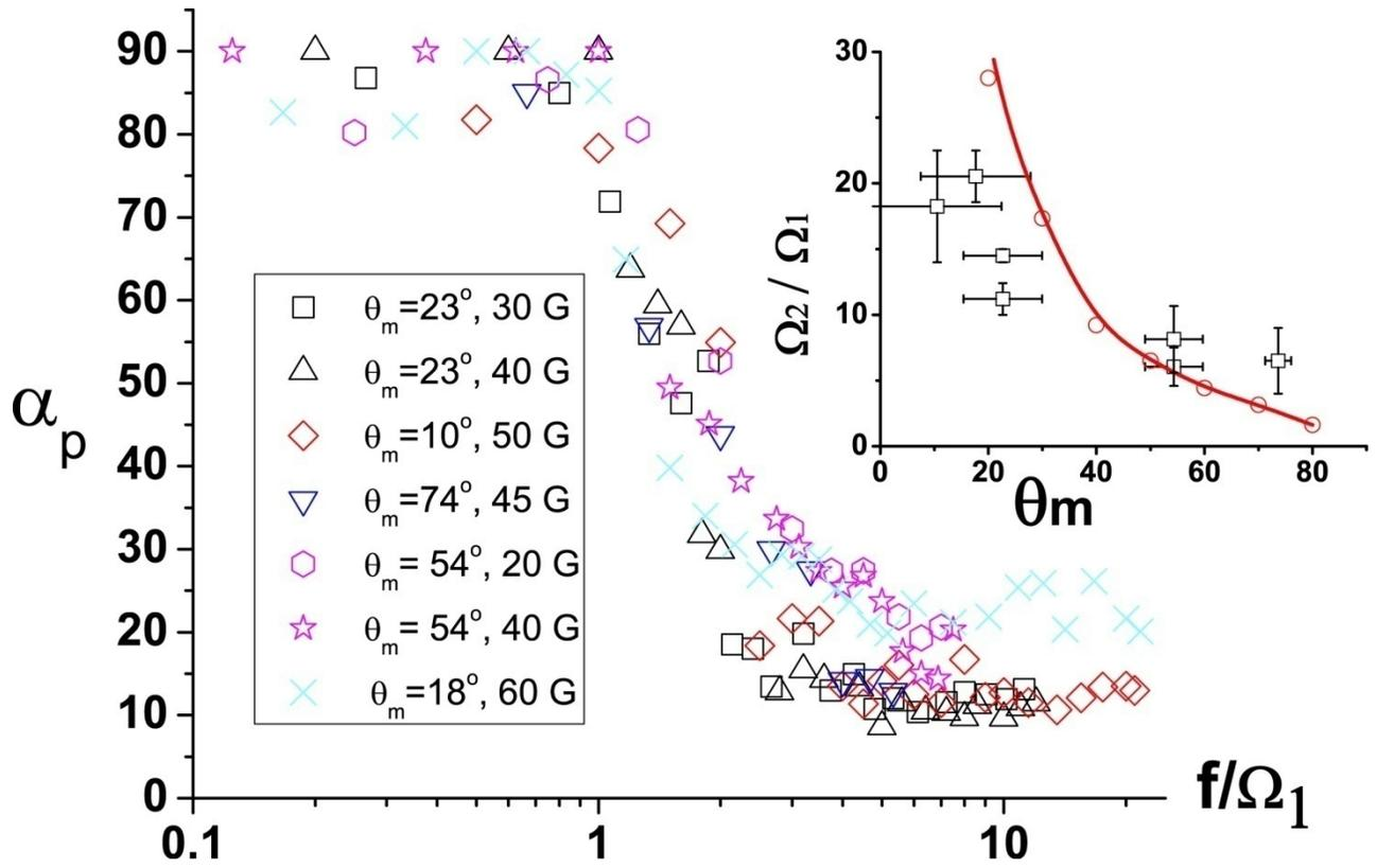
Figure 3 (color online): Variation of the precession angle as a function of the scaled frequency for propellers with various directions of magnetization under different magnetic fields. The data is plotted till  $\Omega_2/\Omega_1$ , which varies for the different  $\theta_m$ . (Inset) shows the variation of  $\Omega_2/\Omega_1$  as a function of the angle of magnetization (experimental data: squares, simulation: circles and solid line).
