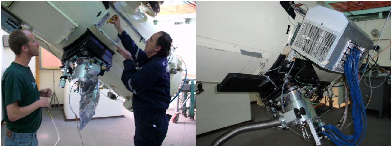
Fig. 4.— Left: Installation of the PreCam instrument on the University of Michigan Curtis-Schmidt telescope at CTIO. Right: A close-up of the PreCam instrument fully installed, with associated DAQ electronics connected to the Vacuum Interface Board for data readout.
