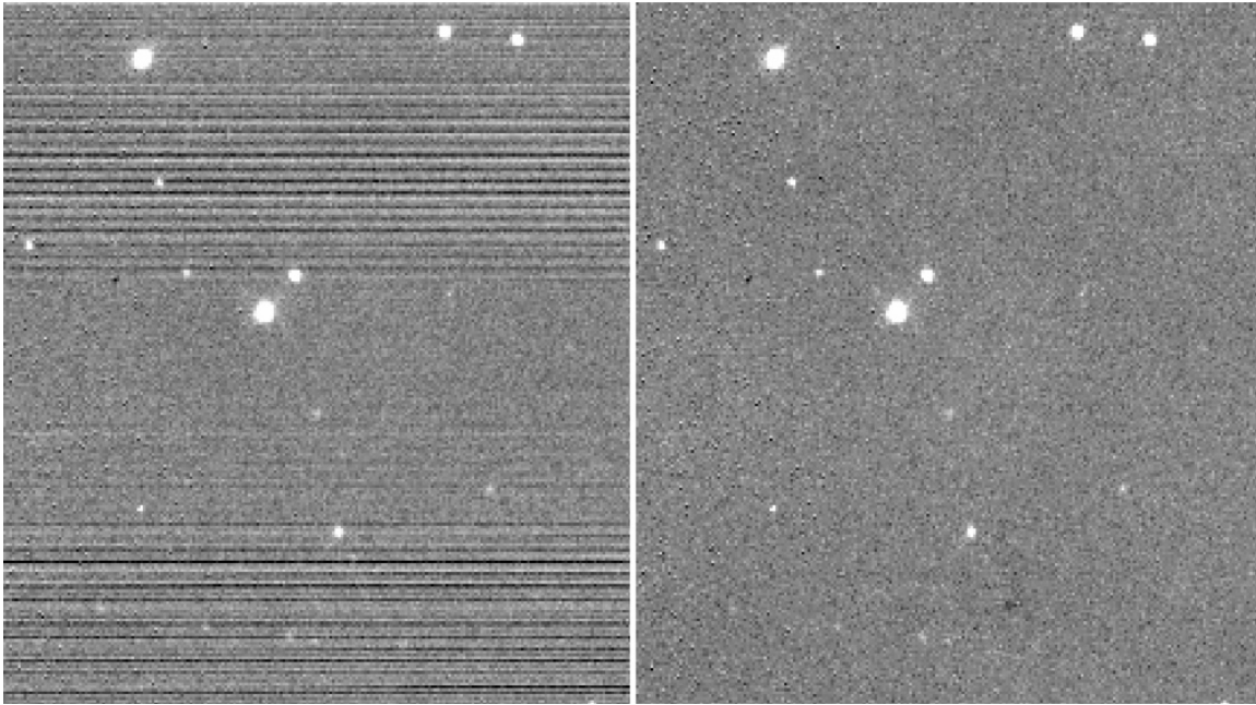
Fig. 10.— Left: A representative PreCam image with significant streaking that would interfere with the photometric determination of the stars in that field. Right: The same image after streaking removal, exhibiting desired behavior for both background regions and stars.
