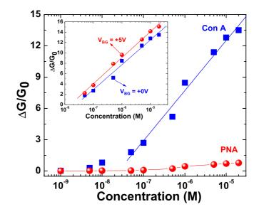
Fig.2.  $\Delta G/G_0$  of the device (a) after adding 2 µL of lectin solution of different concentrations on the SWNT + DM complex. Inset:  $\Delta G/G_0$  vs concentration of con A, fitted using Eq. (1), at  $V_{BG} = 0$  and  $V_{BG} = +5$  V.
