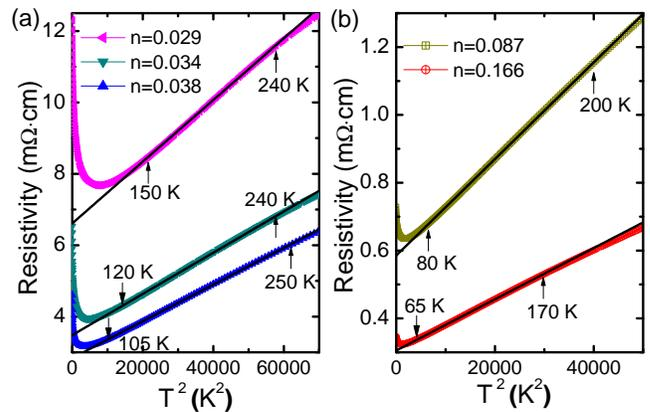
FIG. 3:  $\rho_{ab}$  of  $n$ -type samples as a function of  $T^2$  for the same data shown in fig. 2. Solid line is the fitting to the data. Arrows indicate the  $T$  where  $\rho_{ab}$  deviates from Fermi-liquid behavior.
