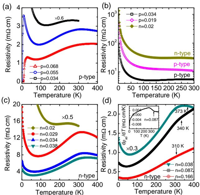
FIG. 2: The in-plane resistivity  $\rho_{ab}$  as a function of temperature for  $p$ -type and  $n$ -type thin films. The samples were labeled by the hole ( $p$ ) and electron ( $n$ ) doping at 300 K (per Cu atom) which is obtained by Hall measurement. Inset of (d) is the temperature derivative of  $\rho_{ab}$  for sample with  $n=0.087$ .
