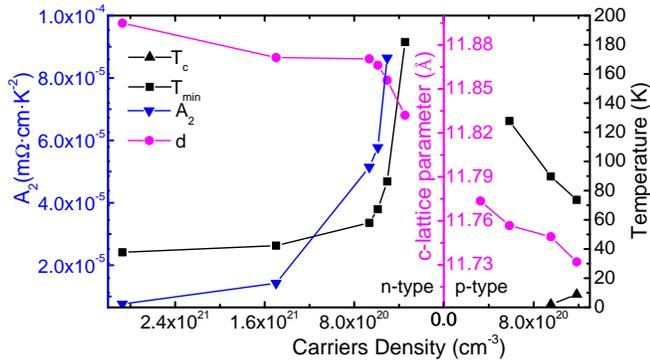
FIG. 5: Superconductivity transition temperature  $T_c$ , temperature with minimum resistivity  $T_{min}$ ,  $c$ -lattice parameter  $d$  and quadratic scattering rate  $A_2$  as a function of carriers density at 300 K.  $T_{min}$  is obtained by calculating the derivatives  $d\rho_{ab}/dT$  and is the temperature when  $d\rho_{ab}/dT=0$ .  $A_2$  is obtained from fitting  $\rho_{ab}(T)=\rho_0+A_2T^2$  to data within  $\rho_{ab}\propto T^2$  region shown in fig.3.
