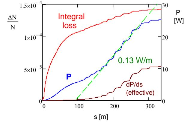
Figure 3. Integrals over linac length for the relative particle loss rate and the power density due to particle loss.
