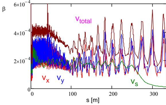
Figure 2. Transverse and longitudinal rms velocities ( $\beta = v/c$ ) along the SNS linac extracted from numerical simulations;  $\varepsilon_{nx}/\varepsilon_{ny} = 0.22/0.25 \text{ mm mrad}$ ,  $\varepsilon_s = 0.9 \text{ eV } \mu\text{s}$ .
