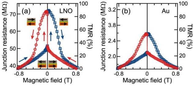
FIG. 4. Comparison of TMR curves of (a) LNO/PCMCO ( $y=0.2$ ) (10 ML)/STO (2 ML)/LSMO and (b) poly-Au/PCMCO ( $y=0.2$ ) (10 ML)/STO (2 ML)/LSMO junctions measured at 4 K under a bias voltage of -5 mV. The scan direction is indicated by red and blue arrows in (a).
