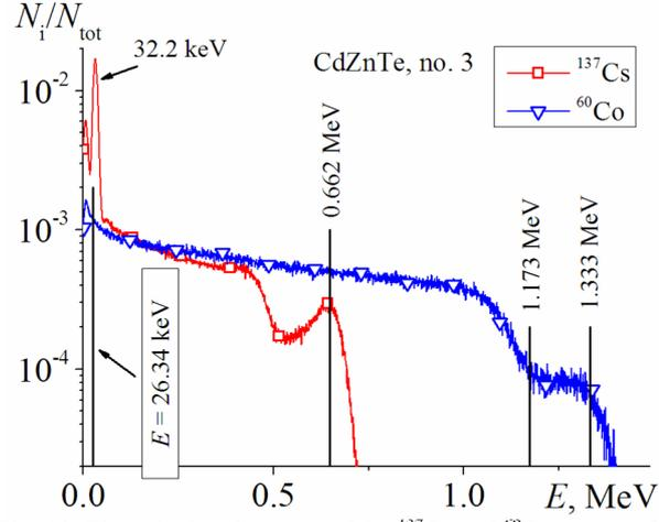
Fig. 10. The calculated spectra of the  $^{137}\text{Cs}$  and  $^{60}\text{Co}$  sources for CdZnTe detector.
