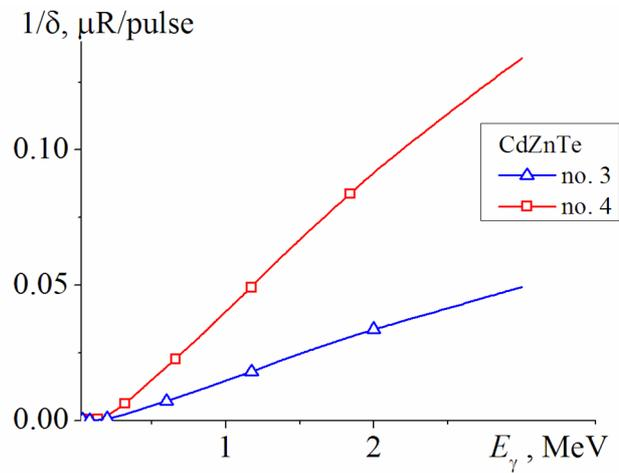
Fig. 8. The dependence  $1/\delta = f_0(E_\gamma)$  for CdZnTe detectors.
