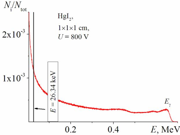
Fig. 5. The change of HgI<sub>2</sub> detector response at the bias reduction.
