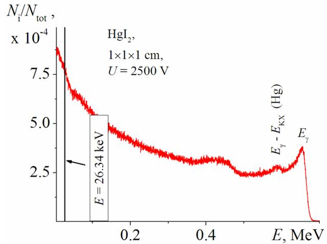
Fig. 4. The response of HgI<sub>2</sub> detector after the output of the measuring channel corresponded to Ref. [20].
