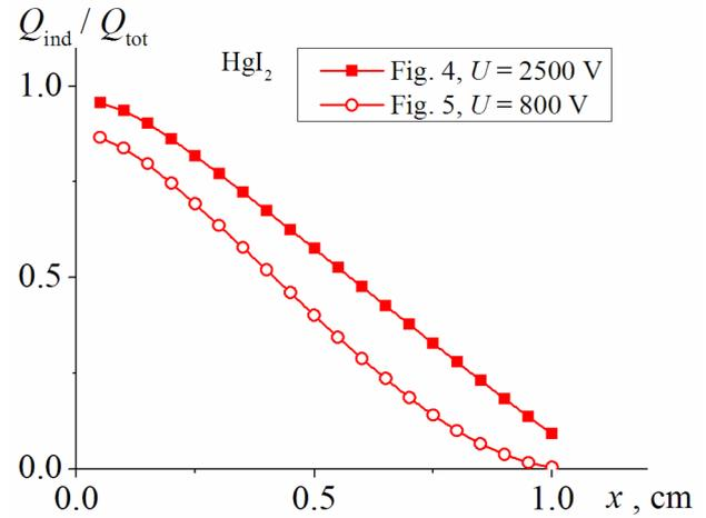
Fig. 6. The change of the charge collection efficiency  $CCE(x)$  in the HgI<sub>2</sub> detector.
