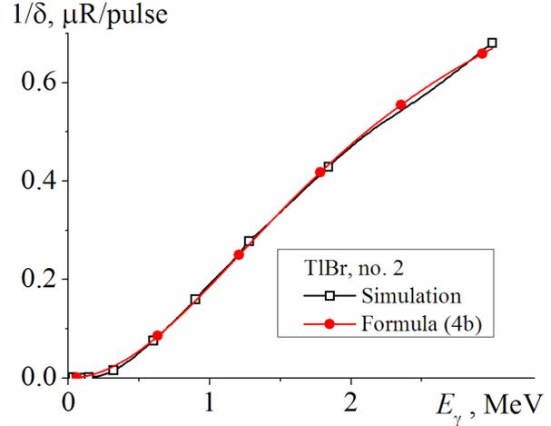
Fig. 17. The total  $1/\delta$  dependence for TlBr detector.
