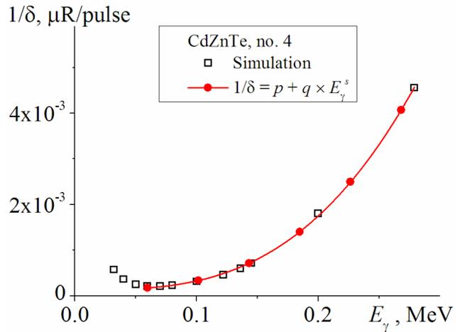
Fig. 12. The fitting of the dependence  $1/\delta$  using the power function for CdZnTe detector ( $p$ ,  $q$ ,  $s$  – fitting parameters).
