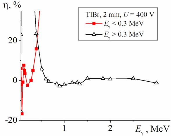
Fig. 19. The difference between the approximate  $1/\delta$  calculation with formulas (4) and the Monte-Carlo simulation data for TlBr detector with the thickness of 2 mm.
