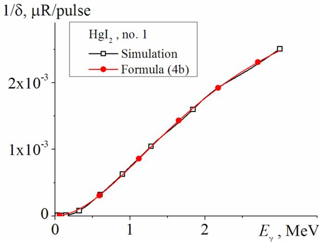
Fig. 14. The  $1/\delta$  dependence for HgI<sub>2</sub> detector.
