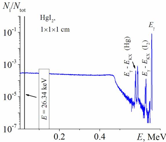
Fig. 3. The response function of HgI<sub>2</sub> detector on gamma-quanta with energy 662 keV without taking into consideration the charge collection and noises.
