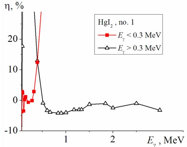
Fig. 15. The difference between the approximate formulas (4) for calculation of  $1/\delta$  and the Monte-Carlo simulation data for HgI<sub>2</sub> detector.
