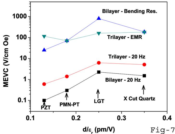
Fig.7: Low-frequency and resonance MEVC as a function of the ratio of the piezoelectric coupling coefficient  $d$  to the relative permittivity  $\epsilon_r$  for bilayers and trilayers of permendur and ferroelectric PZT or PMN-PT and piezoelectric LGT or quartz.
