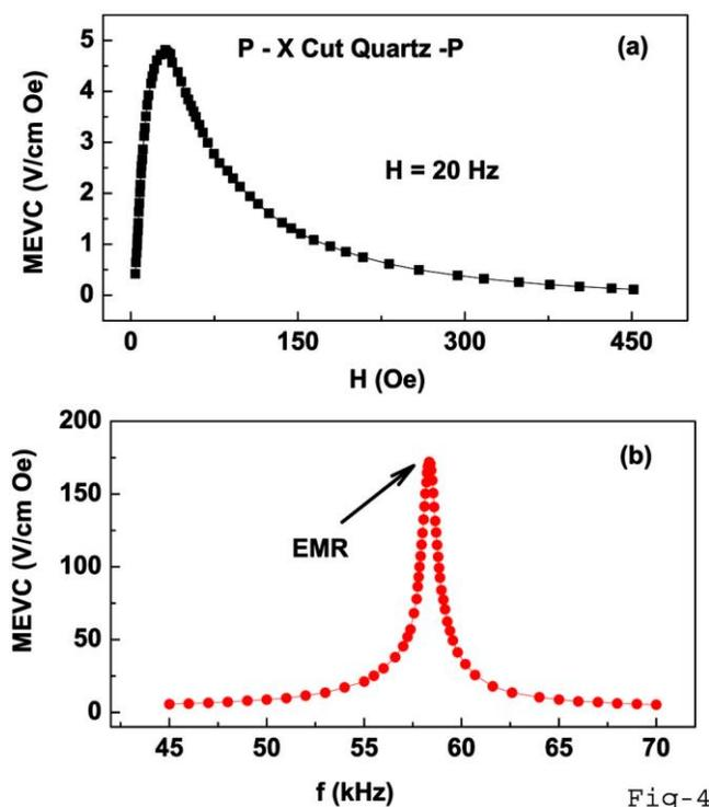
Fig.4: Similar (a) MEVC vs H and (b) MEVC vs  $f$  data for a trilayer of P-X-cut quartz-P. The resonance in Fig.3(b) occurs at electromechanical resonance corresponding to the longitudinal acoustic mode for the trilayer.
