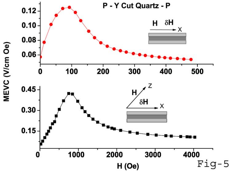
Fig. 5: Low-frequency MEVC vs H data a bilayer of Y-cut quartz and permendur for (a) bias field  $H$  and ac field  $\delta H$  parallel to X-direction and (b)  $H$  along Z-direction and  $\delta H$  along X-direction. Face-shear deformation leads to a strong ME coupling for this case.
