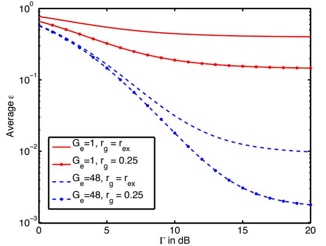
Fig. 3. Outage probability in mixed fading as a function of SNR averaged over 10,000 networks drawn under the same conditions as the one shown in Fig. 1. For each network, shadowing with  $\sigma_s = 8$  dB is applied.
