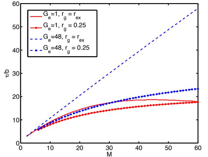
Fig. 6. Transmission capacity as a function of the number of placed mobiles  $M$ . An exclusion zone of  $r_{ex} = 1/12$  is used. Performance is shown both with spreading ( $G_e = 48$ ) and without spreading ( $G_e = 1$ ), and both with a CSMA guard zone ( $r_g = 1/4$ ) and without an additional CSMA guard zone ( $r_g = r_{ex}$ ). The channel model is the same as in Fig. 3 at  $\Gamma = 10$  dB.
