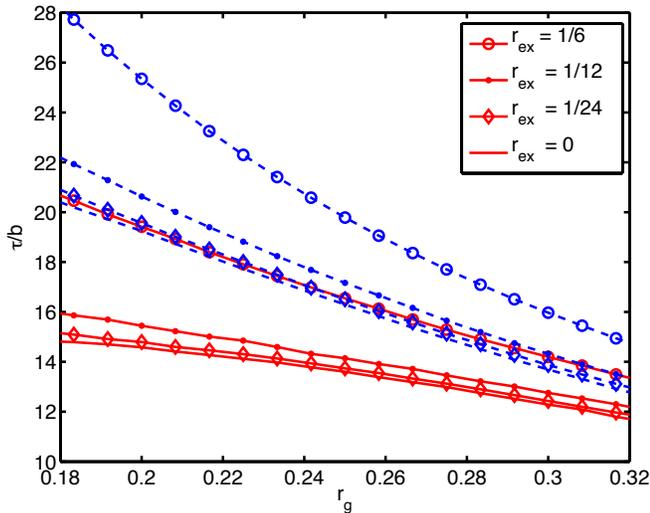
Fig. 5. Transmission capacity as a function of  $r_g$  for several values of  $r_{ex}$ . Dashed lines are with spreading ( $G_e = 48$ ) while solid lines are without ( $G_e = 1$ ). The channel model is the same as in Fig. 3 at  $\Gamma = 10$  dB.
