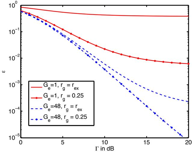
Fig. 2. Outage probability as a function of SNR, conditioned on the network shown in Fig. 1 with mixed fading and no shadowing. Dashed lines are with spreading ( $G_e = 48$ ) while solid lines are without. Curves marked with  $\bullet$  indicate performance with a CSMA guard zone of radius  $r_g = 1/4$  while curves without markers indicate performance without CSMA guard zones.
