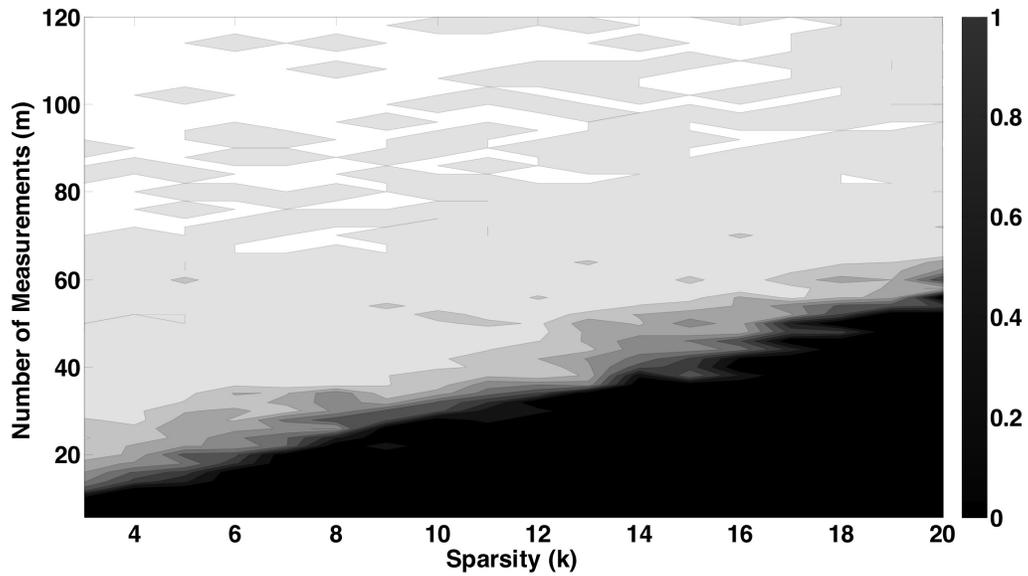
Figure 16. **Approximately sparse signal and noisy measurements – reconstruction performance for fixed signal-length  $n$ :** As in Fig 14, the  $y$ -axis denotes the number of measurements  $m$ , and the  $x$ -axis denotes the sparsity  $k$ , for fixed signal length  $n = 1000$ . In this case, we set  $\sigma_z = 0.03$ , and allowed relative reconstruction error of at most 0.3.
