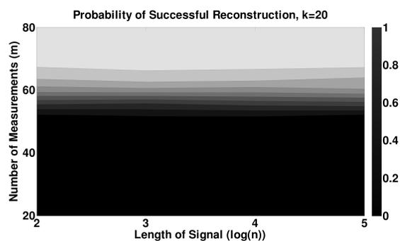
Figure 15. **Exactly sparse signal and noiseless measurements – reconstruction performance for fixed sparsity  $k$ :** The number of measurements  $m$  are plotted on the  $y$ -axis, plotted against  $\log(n)$  on the  $x$ -axis – the sparsity  $k$  is fixed to be 20. Note that there is *no* scaling of  $m$  with  $n$ , as guaranteed by our theoretical bounds.
