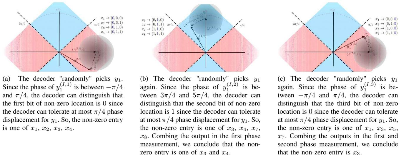
Figure 13. If we were to distinguish each  $j$  from 1 to 8 by a different phase, the decoder can tolerate at most  $\pi/14$  phase displacement for any output  $y_i$ . Instead, we first represent each  $j = 1, 2, \dots, 8$  by a three-length binary vector. Next, we perform three sets of phase assignments – one for each digit. It is easily seen that by allowing multiple measurements, the noise tolerance for the decoder increases.
