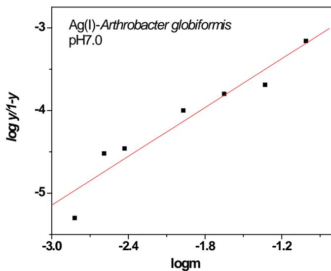
Fig. 2. Biosorption isotherms for Ag(I) - *Arthrobacter oxidas* and Ag(I)- *Arthrobacter globiformis* complex for neutral pH in Hill coordinates.
