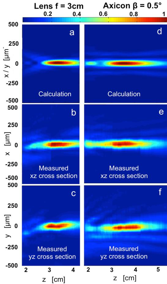
**Fig 3.** a-c) Theoretical calculations and experimental results of the intensity distribution in the focal region for the flat lens with  $f=3\text{cm}$ . a) is calculated using the dipolar model. b and c are the experimental results showing the  $xz$  and  $yz$  longitudinal cross section of the 3-dimensional far-field distributions. d-f) Theoretical calculations and experimental results of the intensity distribution for the planar axicon with  $\beta=0.5^\circ$ .
