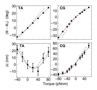
FIG. 3: (Color online) Fitting of analytical models to the results of all-atom MD simulations of two DNA fragments (TA and CG) [7]. Error bars show statistical errors. In the upper two panels the symbol size corresponds to maximal errors. The dashed red lines show the results of fitting for a polynomial torsional potential without a TTC applied. The solid black lines show best fit dependences for a fourth order polynomial with optimized TTC.
