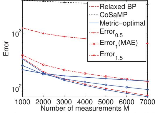
Fig. 4: Comparison of the metric-optimal estimation algorithm, relaxed BP, and CoSaMP. The “MAE” and the “Error<sub>1.5</sub>” lines for “CoSaMP” appear beyond the scope of vertical axis. (Sparse Weibull input and Poisson channel; sparsity rate = 3%; input length  $N = 10,000$ ; input scaling factor  $\alpha = 100$ .)
