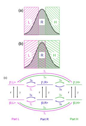
Figure 5: (a) Situation corresponding to two non-overlapping windows that do not cover the whole line. The central region R is not detected by any of the spectrometers. (b) Situation corresponding to two overlapping spectral windows that cover the whole line. The central part R corresponds here to the overlap region. In this case, the spectral window covered by the first (resp. second) spectrometer is L+R (resp. H+R). (c) Level scheme used for the rate equation model (see text).
