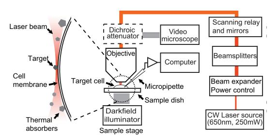
Figure 1. Experiment Block Diagram
