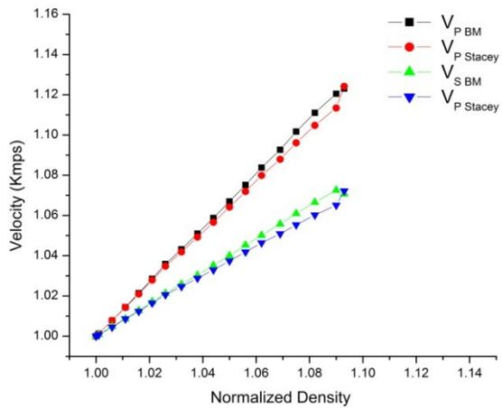
Fig 3. Variation of Reduced velocities with normalized density
