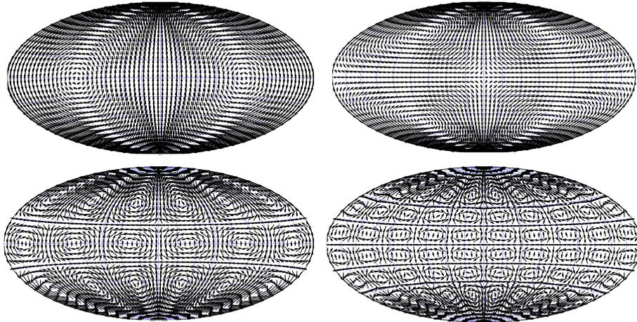
**Fig. 3.** Examples of toroidal harmonics vector fields. From top to bottom and left to right :  $T_{1,1}, T_{2,1}, T_{5,3}, T_{10,5}$ . One sees the change in the angular resolution with larger degrees. The  $T_{1,1}$  is a simple rotation about the  $y$ -axis.
