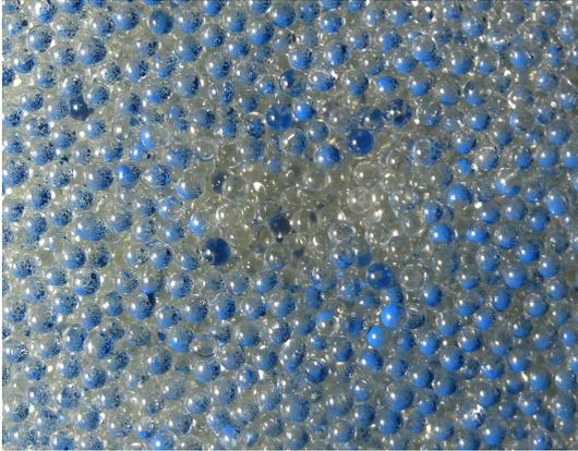
Figure 2: Example for the application of the spray-paint method in shot 27 with 3 mm target grains. The crater is very irregular but the shape can clearly be recognized from the change in color.
