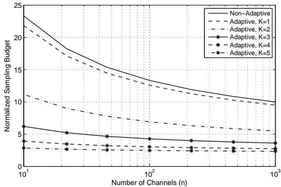
Fig. 2. Average number of observations taken per channel versus the number of channels  $n$ . All the curves correspond to the target error probability for detecting  $T = 2$  holes is  $P_A(n) = P_{NA}(n) = 10^{-4}$ .
